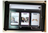
Custom iPad Screen Guards: In collaboration with the Tech Resource Center Marin, a program of the Marin County Office of Education, we are designing and producing acrylic screen guards for use with touch screen monitors. These screen guards are specifically designed to assist physically challenged individuals when using iPads and other touch activated devices.
